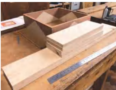
▲ Pic.24 In the meantime I sanded down the door panels using a wide belt sander and rough cut the interior components for the cabinet
